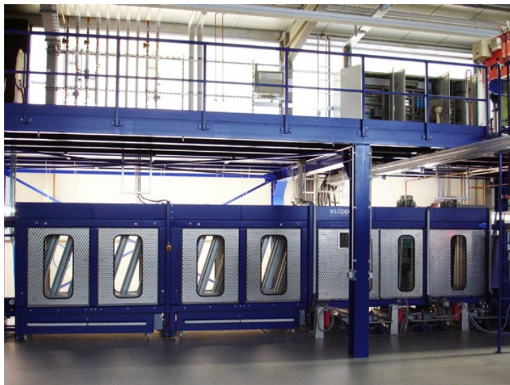
Washing and drying system
