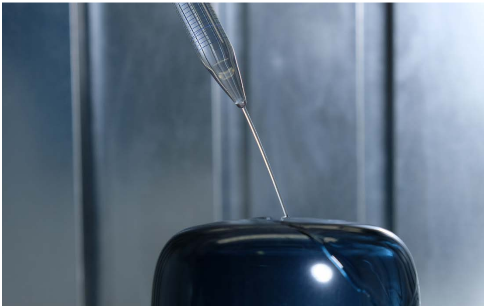
Flow coating of glass
