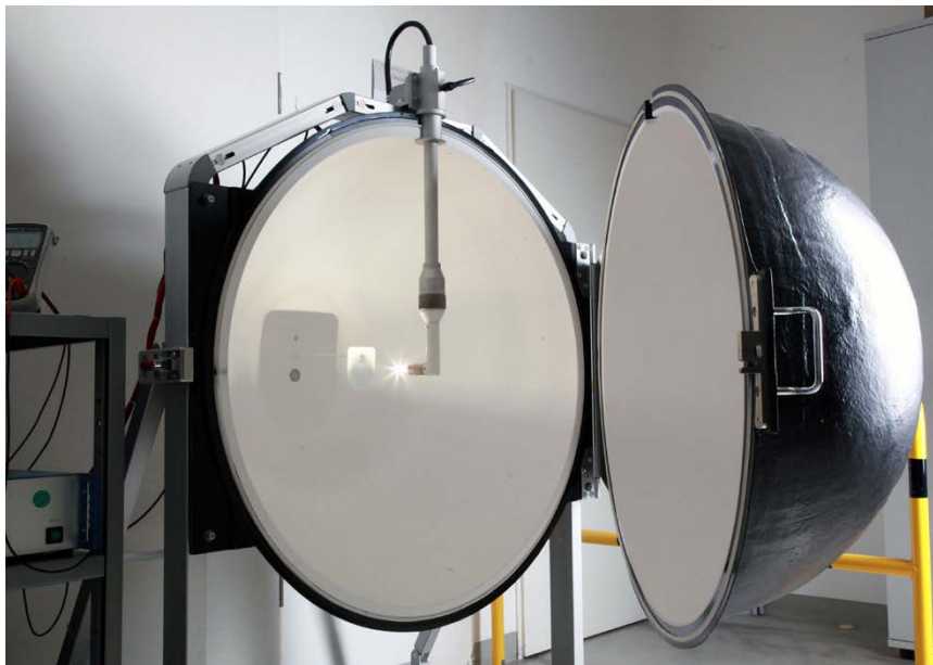
Integrating sphere – 1 m diameter
