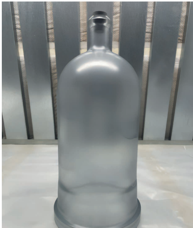
Reactor with shatter protection coating on the outside and additional anti-static coating
