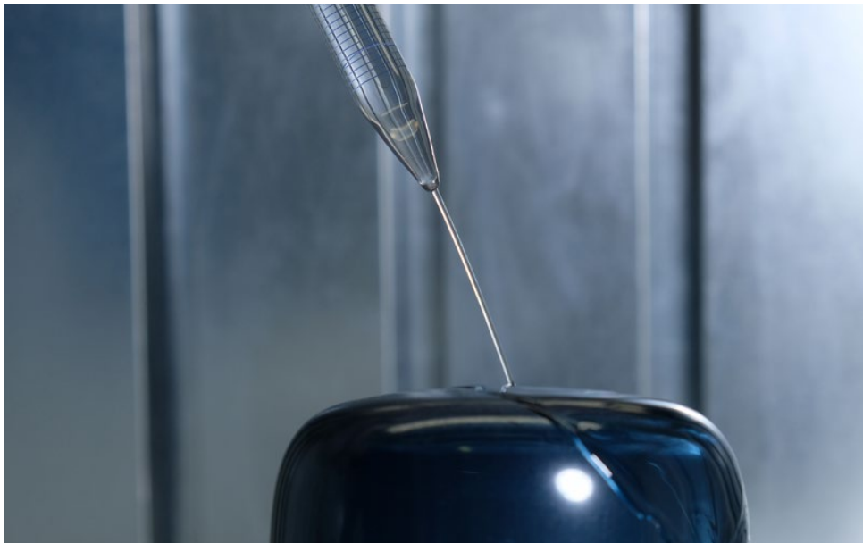
Coating of glass by flooding
